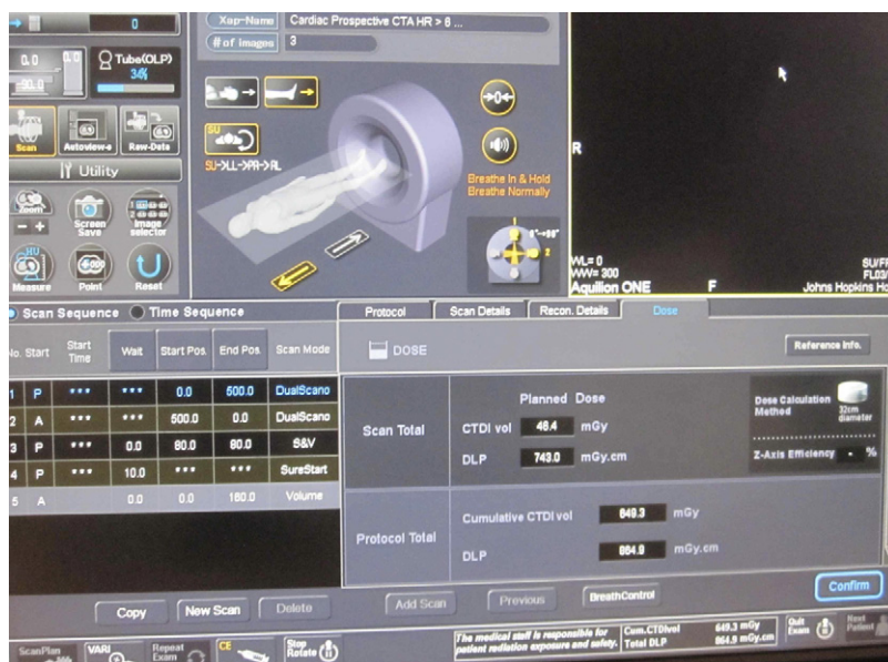
Fig 1. Sample prescan dose display at CT control console displaying volume CT dose index (CTDIvol), dose-length product (DLP) for the chosen protocol, and the type of phantom used in determining CTDIvol (Toshiba Medical Systems, Nasu, Japan).
